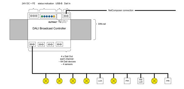
The new DALI Broadcast Controller DBC allows an easy and efficient method of implementing energy-optimized shop floor lighting systems. DALI Light fixtures in large contiguous areas can now easily be addressed by broadcast commands instead of conventional single device-addressing.
